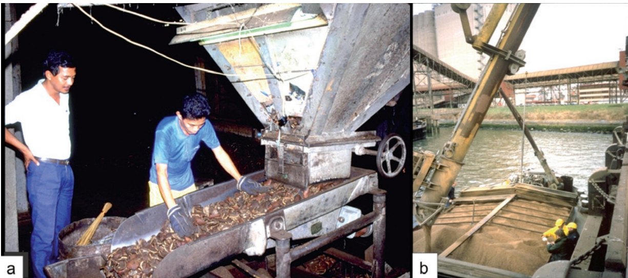
Fig. 3.3. Sampling of mobile batches: (a) copra cake emerging from a hopper; (b) sampling a 500 t batch of oilseed meal as it flows into a barge. Photographs courtesy of Raymond Coker, ToxiMet Limited.
