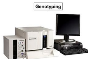
Luminex ➤ Beads are analyzed in the Luminex reader to identify the infectious agents
